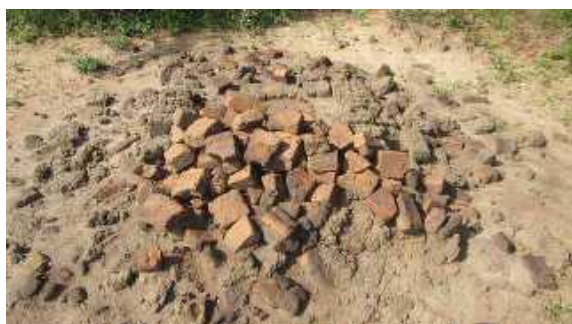
Plate 17-22: Evidence of a failed attempt at brick production in the NGR-02 study area. The use of brick in the study area is extremely rare/non-existent due to the lack of suitable raw materials.
