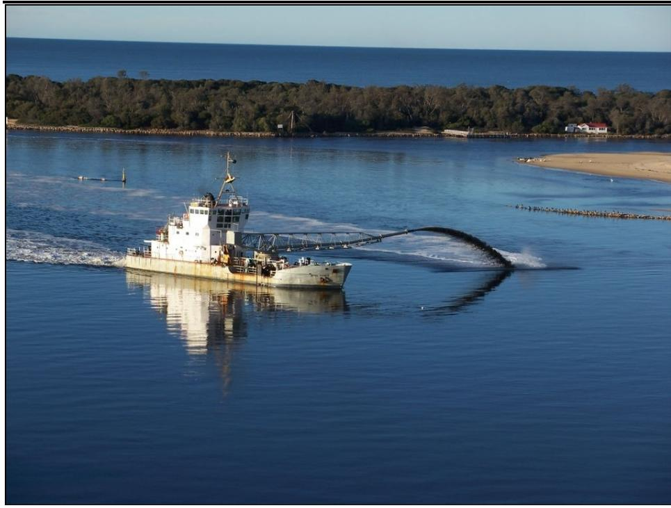
*Figure.4 Typical TSHD (material stored on board for disposal at appropriate location)*
